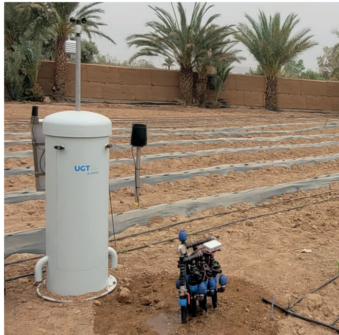
Soil Hydrological Measuring Station, project SuLaMo, Morocco
